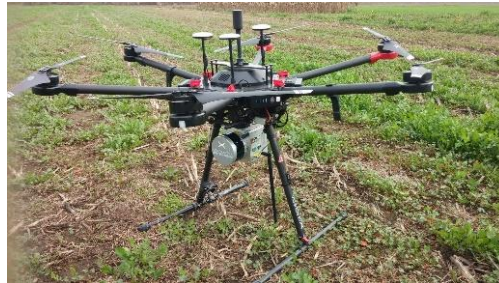
Figure 4 – The LiDAR data acquisition system
